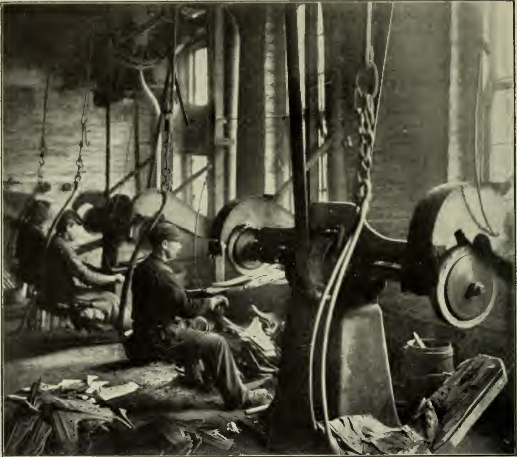
CARBORUNDUM WHEELS AT WORK ON CHILLED IRON PLOUGH POINTS.
